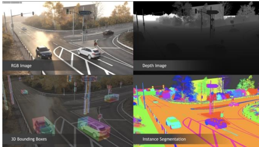
Figure 3- NVIDIA Drive Sim being used to gather data that will be used to train neural networks for autonomous vehicle perception
