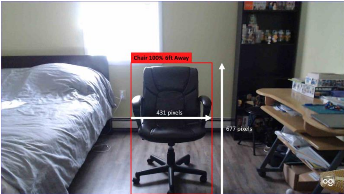
Figure 5: Chair measured to be 6ft away (431 pixels wide and 677 pixels tall in frame)
