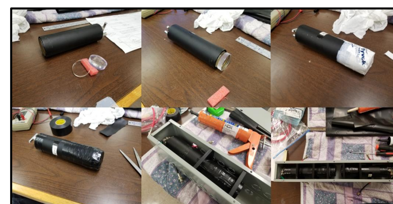
Figure 7. Assembling the BC-408 scintillation counter and installing it into the prototype housing. The NaI(Tl) scintillation counter was assembled in a similar process. Both are shown in the housing at bottom right. Brackets were custom-designed and 3d printed.
