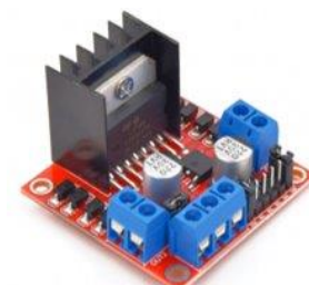
Figure 3. Arduino Motor Controller (L298N)
